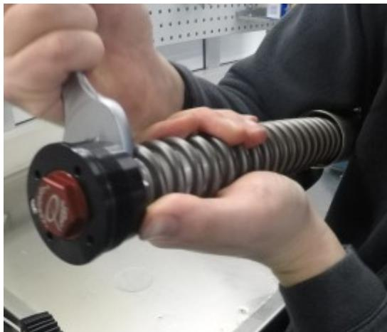
13) Tighten the cartridge cap on the 12 mm rod
