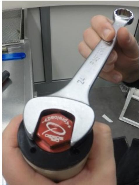
17) Regulate the spring preload with the desired load
