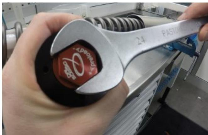
12) Completely unscrew the hexagon spring preload
