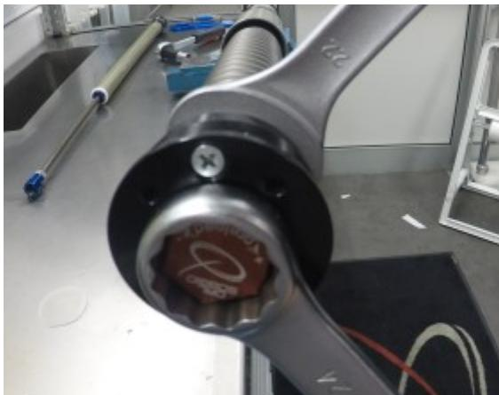
14) Close the locknut and the withe spring spacer on the cartridge cap
