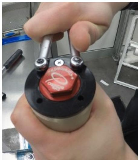
16) Close the cartridge cap on the sheath
