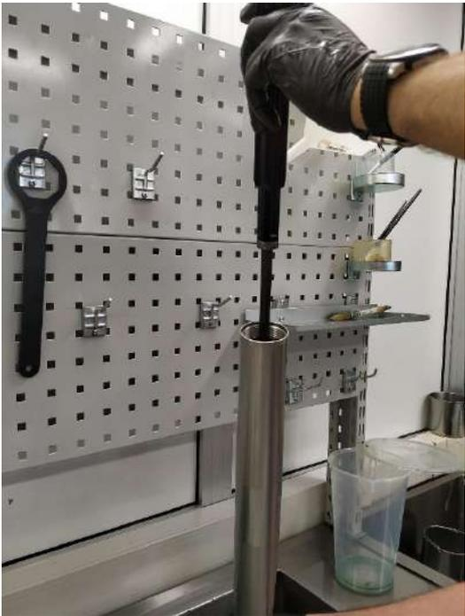
6 - Lock the rod with Stem clamp  $\varnothing$  12 and unscrew the spring guide
