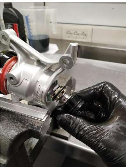
18 - Put the Cube oil on the fork and charge the pumping
