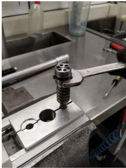
11- Apply the Loctite 243 on rebound holder and fix it on the damper rod with wrench 17
