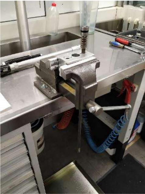
10 – Heat up (not excessively!) the upper part of the rod to soften the Loctite, but pay attention to not ruin the spring's protection in plastic.
