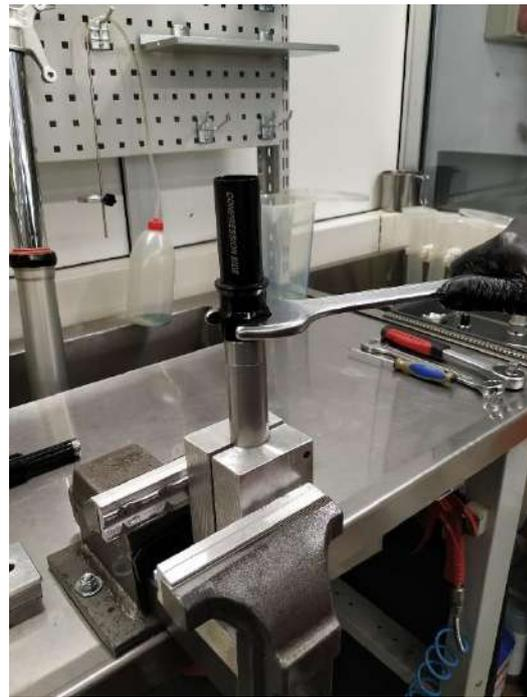
14 – Put the rod that you have previously assemble on the damper tube
