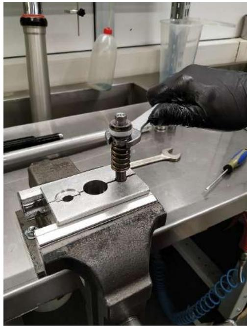
12 - Reinsert the rod previously assembled on inner tube
