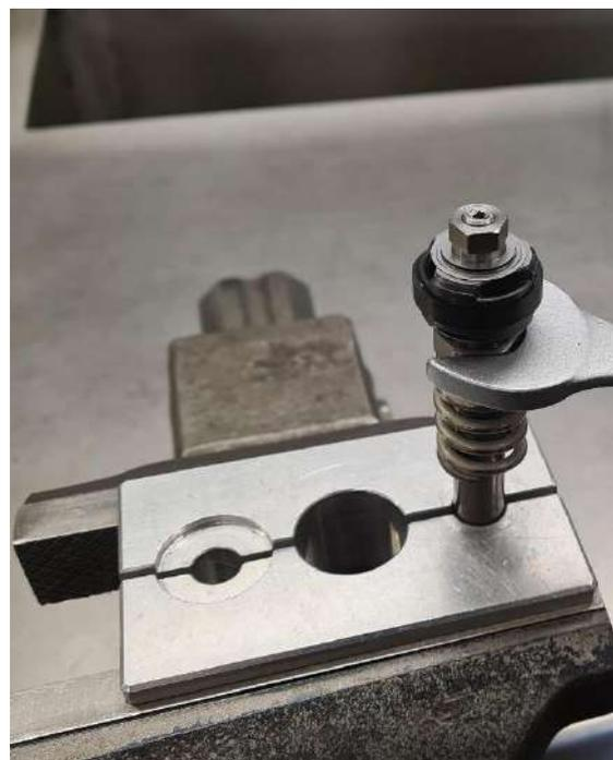
11 - Apply the Loctite 243 on rebound base valve and clamp it on the damper rod with wrench 17
