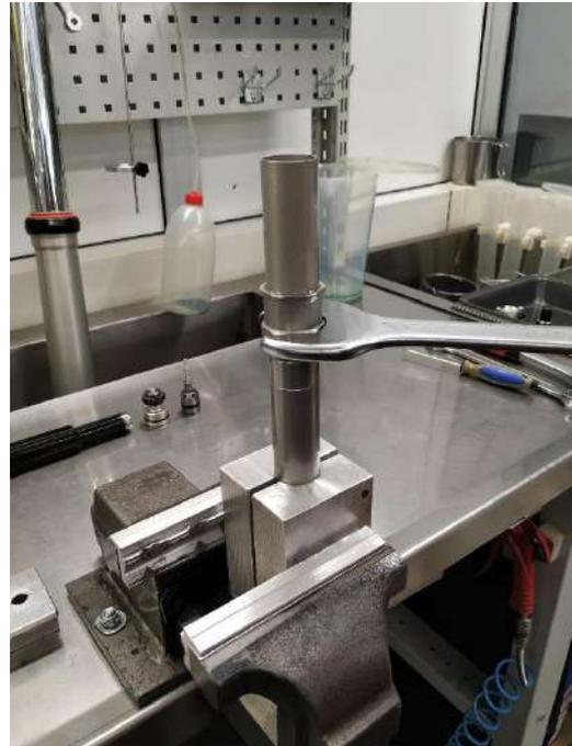
13 – Put the Loctite 243 on damper tube and screw the hydrostop that you find on the kit with wrench 32
