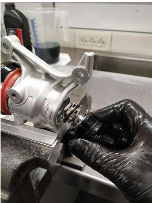
20 – Put the Cube oil on the fork and load the pumping with alternating movements on the entire stroke up to the max extension
