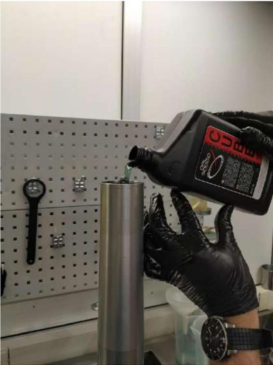
21 – Set up the recommend oil level with the specific tool like in picture below, with tube and  $\varnothing 12\text{mm}$  rod completely lowered.
