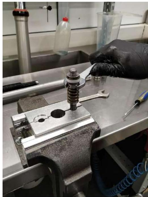
12 – Once removed the plastic cup, heat up the tube near the hydrostop (like in the picture) and unscrew the hydrostop cap with wrench 32
