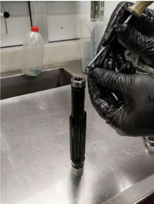
9 – Pull out the damper rod and vise it on clamp  $\varnothing 12$
